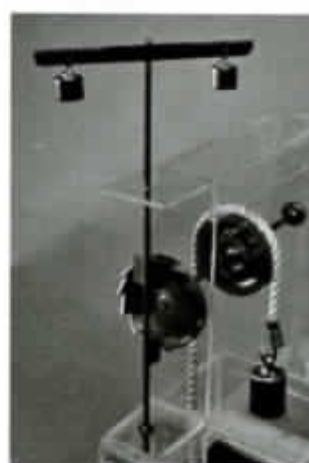
Model of early escapement. Work of Minesaki Sougo. This escapement consists of a crown wheel (a wheel with inclined teeth), a "verge" with two "pallets" (pegs), and a "foliot" (balance) with two adjustment weights. Two pallets are moved right and left by the crown wheel. The oscillating speed of the foliot on the top of the verge is controlled by changing the position of the adjustment weights. The crown wheel is driven by the weights connected to a rope hanging on a wheel, which has a gear and a ratchet inside it. The early European clocks used this kind of escapement system and it is thought to have been invented in the latter half of the thirteenth century.
